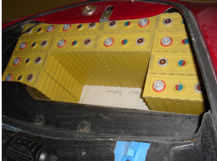
Test fitting 71mm cells (form factor A) into the front battery box
